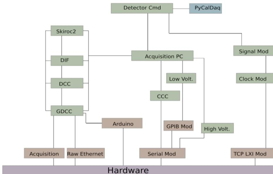
**Figure 6.** Global control-command architecture.
