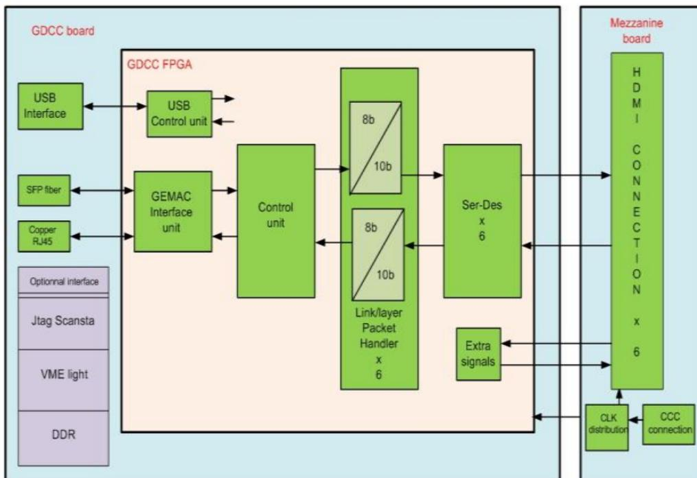
Figure 4. Architecture of the GDCC FPGA.
