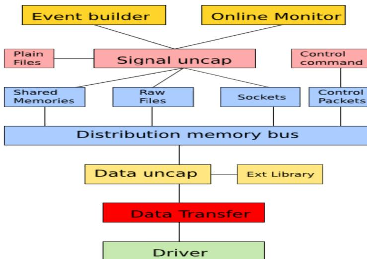
Figure 5. Acquisition chain, software architecture.
