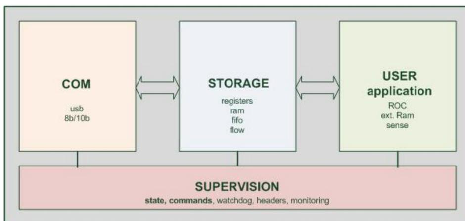
**Figure 2.** Simplified architecture of the DIF FPGA.
