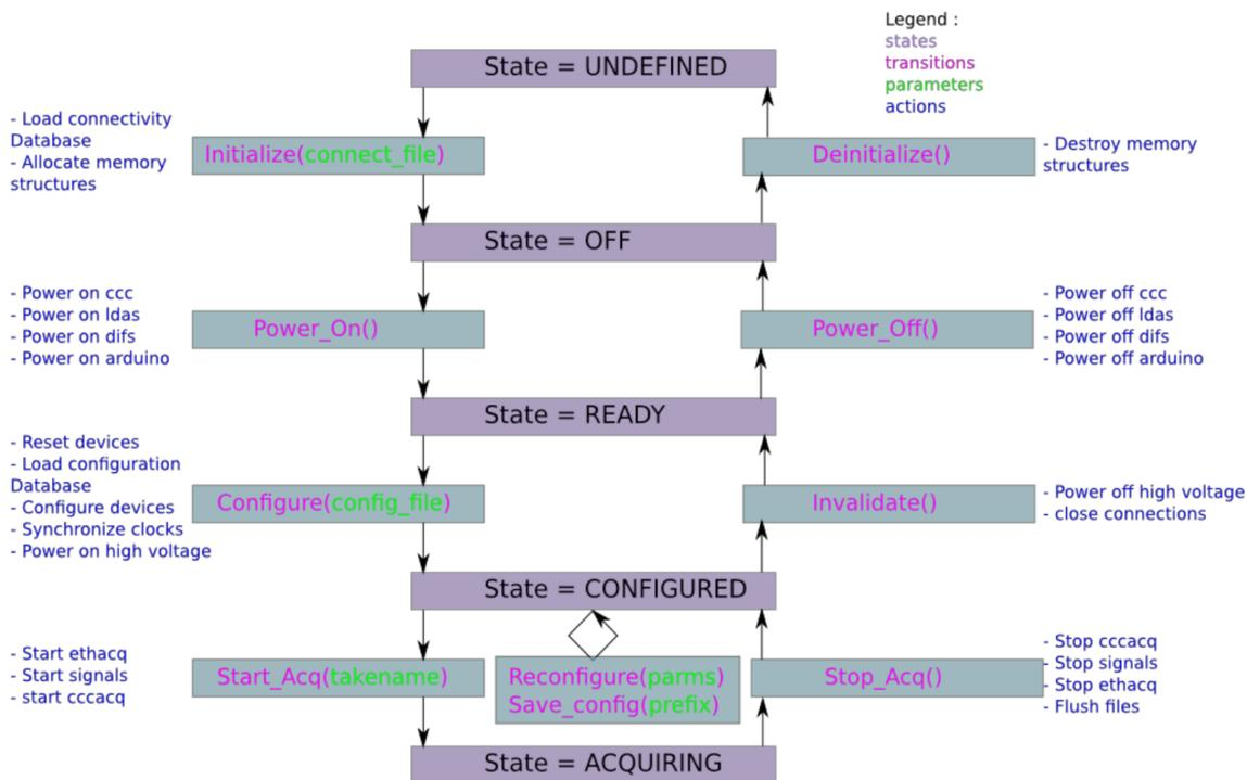
Figure 7. State machine of the detector control-command.
