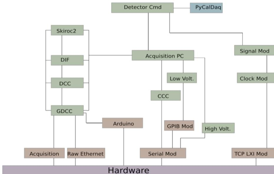
**Figure 6.** Global control-command architecture.
