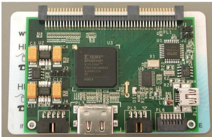
**Figure 1.** Picture of the DIF for the SiW-Ecal.
